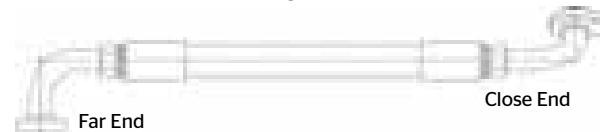
Far End Reference Measuring Clockwise
