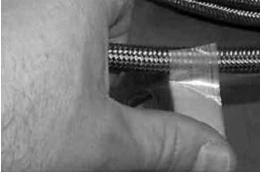
Tape hose before cutting.
